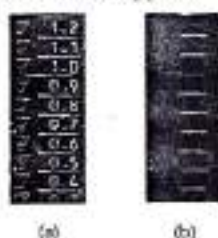
Figure 5. (a) Binary image applied adaptive threshold (b) Scale extraction image by erosion
