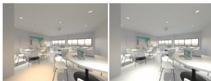
Figure 11: Mix Natural-Spot-Warm lighting (MixNSWL) and Mix Natural-Spot-Daylighting (MixNSDL)
