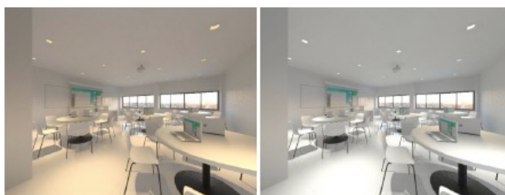
Figure 10: Mix Natural-Spot-Warm lighting (MixNSWL) and Mix Natural-Spot-Daylighting (MixNSDL)
