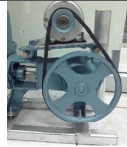
Fig.7. A motor pulley was interlocked with a water pump pulley
