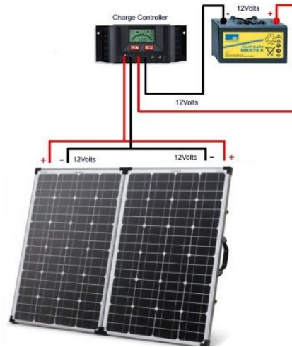
Fig.4. The components for electricity generation from solar energy and a battery charge controller
