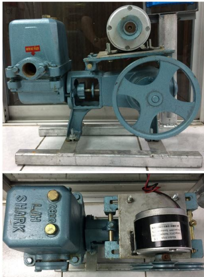
Fig.6. Aluminum sheet and DC motor installed on the water pump
